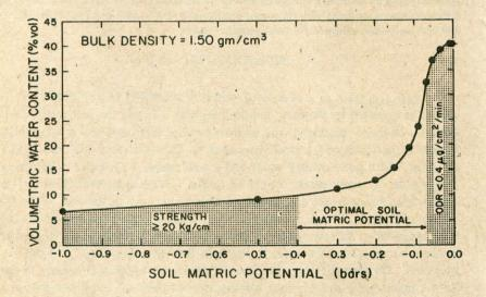
Figure 1. Water desorption, ODR, and strength limiting soil matric potentials of a sandy loam soil /adapted from Phene, 1974/
