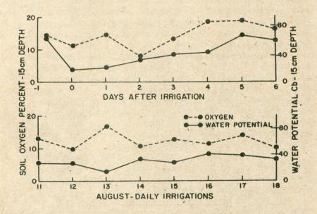
Figure 2. Soil water potential and soil oxygen comparisons for weekly and daily drip irrigation treatments on silty clay loam with watermelon production /Meek, unpublished data/.
